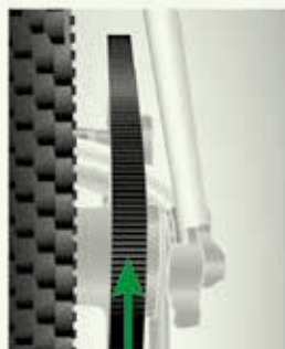
Fig. 45. Correct alignment @Gates
