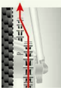
Fig. 46. Sprockets are not aligned correctly @Gates
